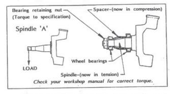
If on the other hand, you fit the standard factory wheel bearing set up, complete with the spacer, tabwasher and wheel bearing retaining nut, tightened to the recommended torque, you will have placed the
